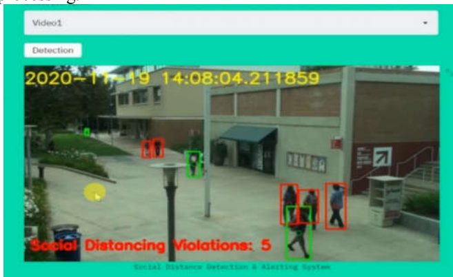
Fig.6. Illustration of Covid-19 Social Distance Detection and Tracking from CCTV videos outputs
