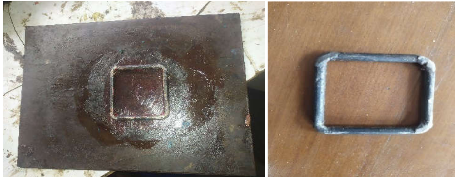
Figure 1: Fabricated mold and spacer
